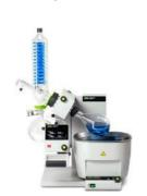
A rotary evaporator is a device used to efficiently remove solvents from samples by evaporation. It distills volatile solution by heating and increasing surface area for distillation. The rotary evaporator is usually connected from a vacuum pump to create vacuum and thus decreases the solution's boiling point.
