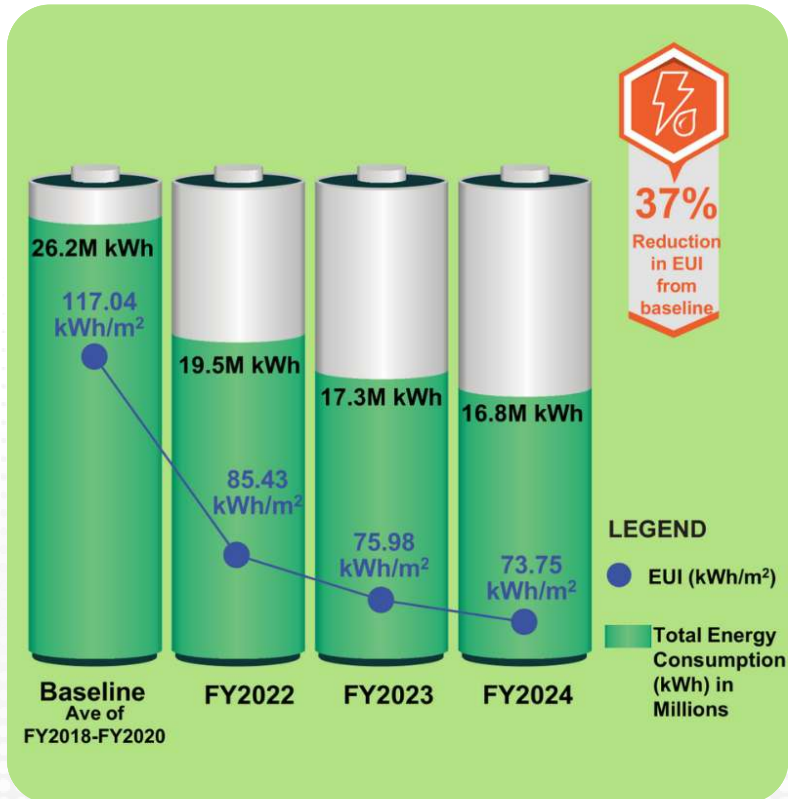
Figure 6 - Total Electricity Consumption & EUI
